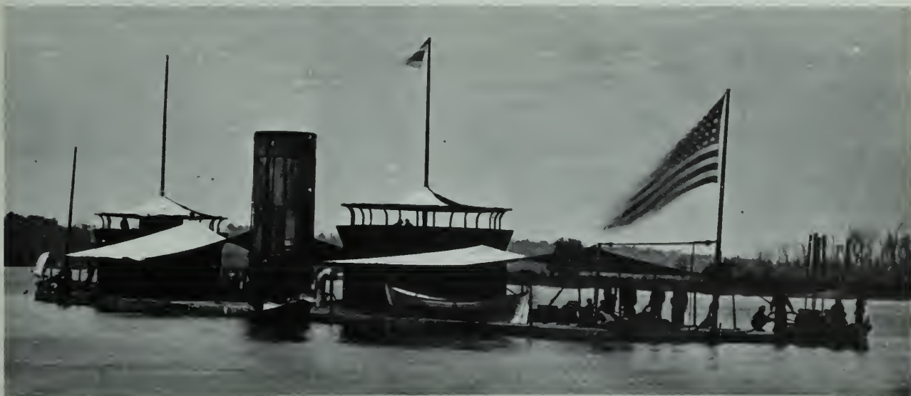
USS Onondaga on the James River during the Civil War—The bulletproof shields installed around the tops of the turrets on many monitors during 1863–65 are clearly visible.
